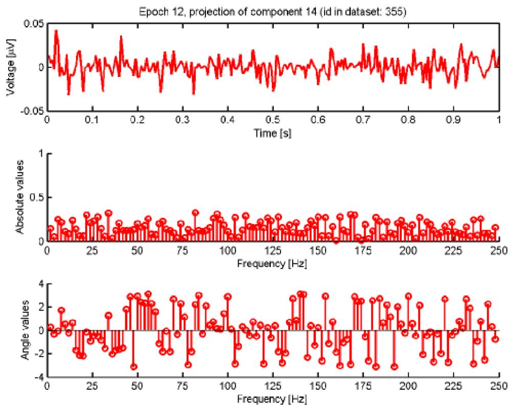
Figure 3.4 Fourier Transform coefficients of artifact signal, adjusted view
