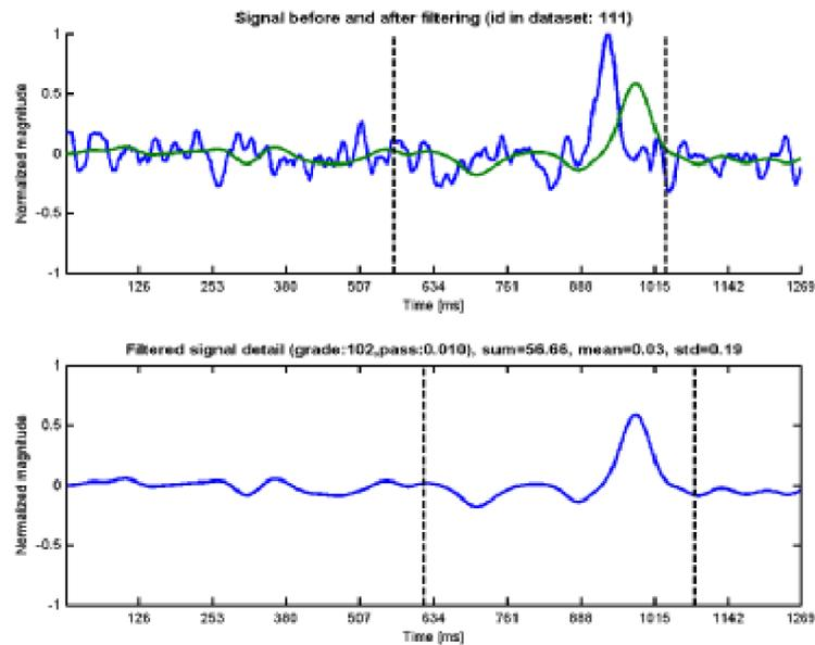
Figure 3.13 The ERP signal identified by FIR filtering method. The vertical lines define the interval of interest. Blue color in the upper part denotes original signal as the green color shows its filtered variation. Lower plot shows the filtered version only with its shifted interval of interest used for computation of statistical methods, which are present in its title.
