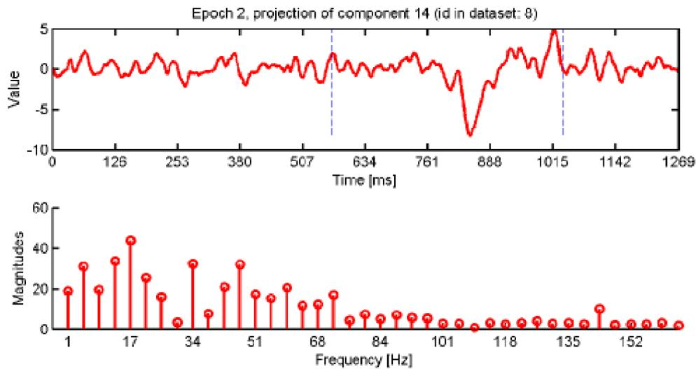
Figure 3.10 FFT absolute coefficients of the ERP signal from real dataset. FFT was applied on the signal within blue vertical line borders only. The significant negative peak starting at time about 700 ms is not reflected in FFT.
