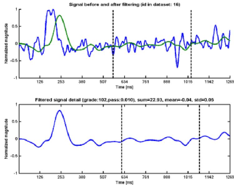
Figure 3.12 The signal rejected based on the FIR filtering method. The vertical lines define the interval of interest. Blue color in the upper part denotes original signal as the green color shows its filtered variation. Lower plot shows the filtered version only with its shifted interval of interest used for computation of statistical methods, which are present in its title.
