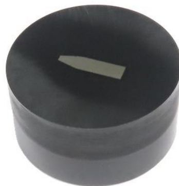
Figure 46 Prepared specimen mounted in resin
