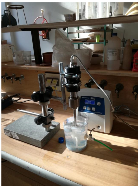
Obr. 41 – Ultrazvuková dispergace nanosiliky
