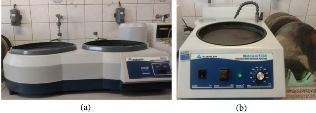
Figure 13: (a) Buehler 2 speed grinder-polisher, (b) MetaServ® 3000 variable speed grinder-polisher
