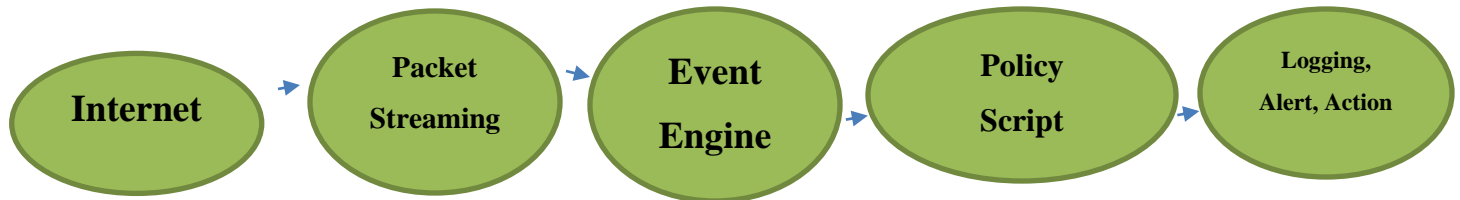
Figure 3: Bro Intrusion Detection system Components
