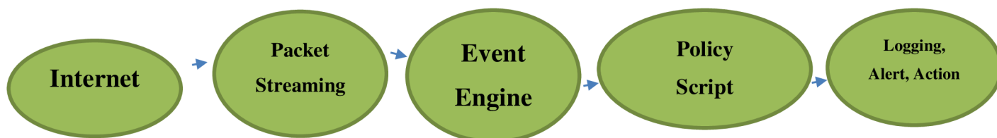
Figure 3: Bro Intrusion Detection system Components
