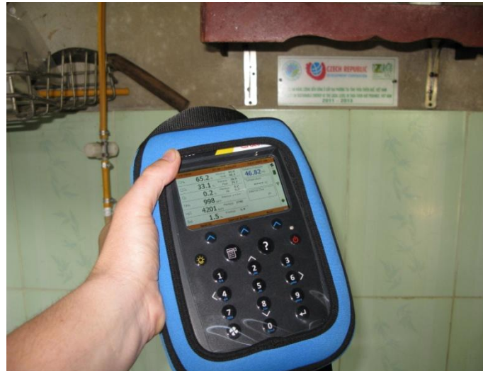
Fig. 3.2: Gas analyzer Geo Tech GA 5000
