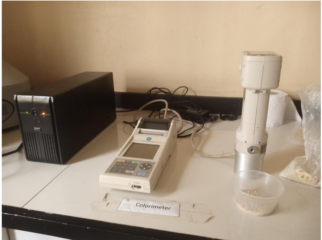
Appendix 5. Chroma Meter (CR-410) colorimeter used for grain colour analysis.
