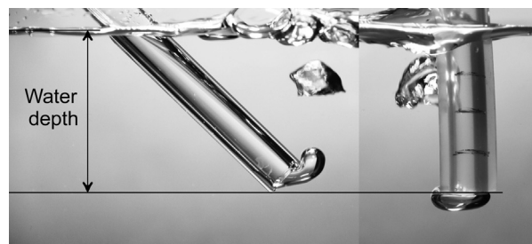
FIGURE 3. Definition of water depth. The resonance tube was used at an angle of 45^\circ (left) and the silicone tube at 90^\circ (right) with respect to the horizontal plane.
