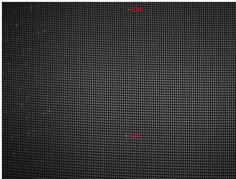
FIGURE 6.2: VIPA spectrum of the unfiltered frequency comb mixed with the diode laser. Each column of dots represents one order of the VIPA etalon transmission. Adjacent orders of transmission are shifted in the vertical direction by 53 GHz to each other and dispersed in the horizontal direction by the diffraction grating. The diode laser mode can be seen in the middle part of the image as two bright spots. They are in two adjacent columns and 53 rows from each other. The bright dots on the left side comes from the frequency comb laser and are its short lived cw modes caused by small coupling of the diode laser into the frequency comb laser cavity.
