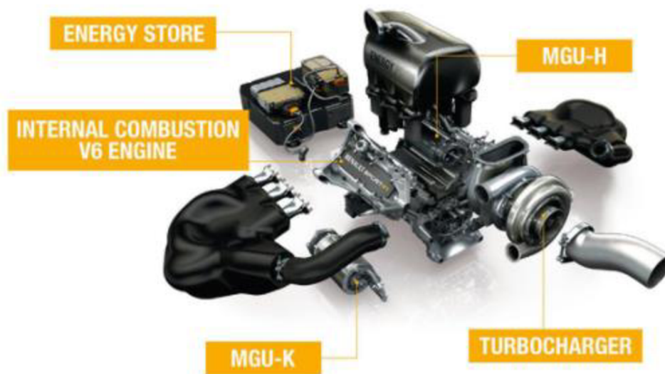
Figure 41 F1 V6 hybrid powertrain with MGU-K and MGU-H generator units for energy recovering [43]
