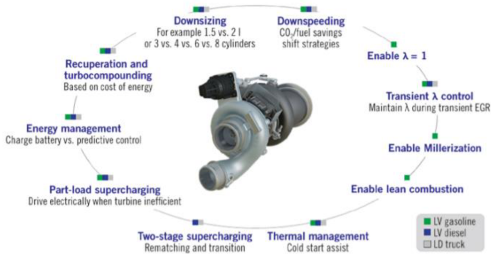
Figure 39 Possible functionalities of an electrified turbocharger for specific applications (Light vehicle gasoline, light vehicle diesel, light duty truck) [41]
