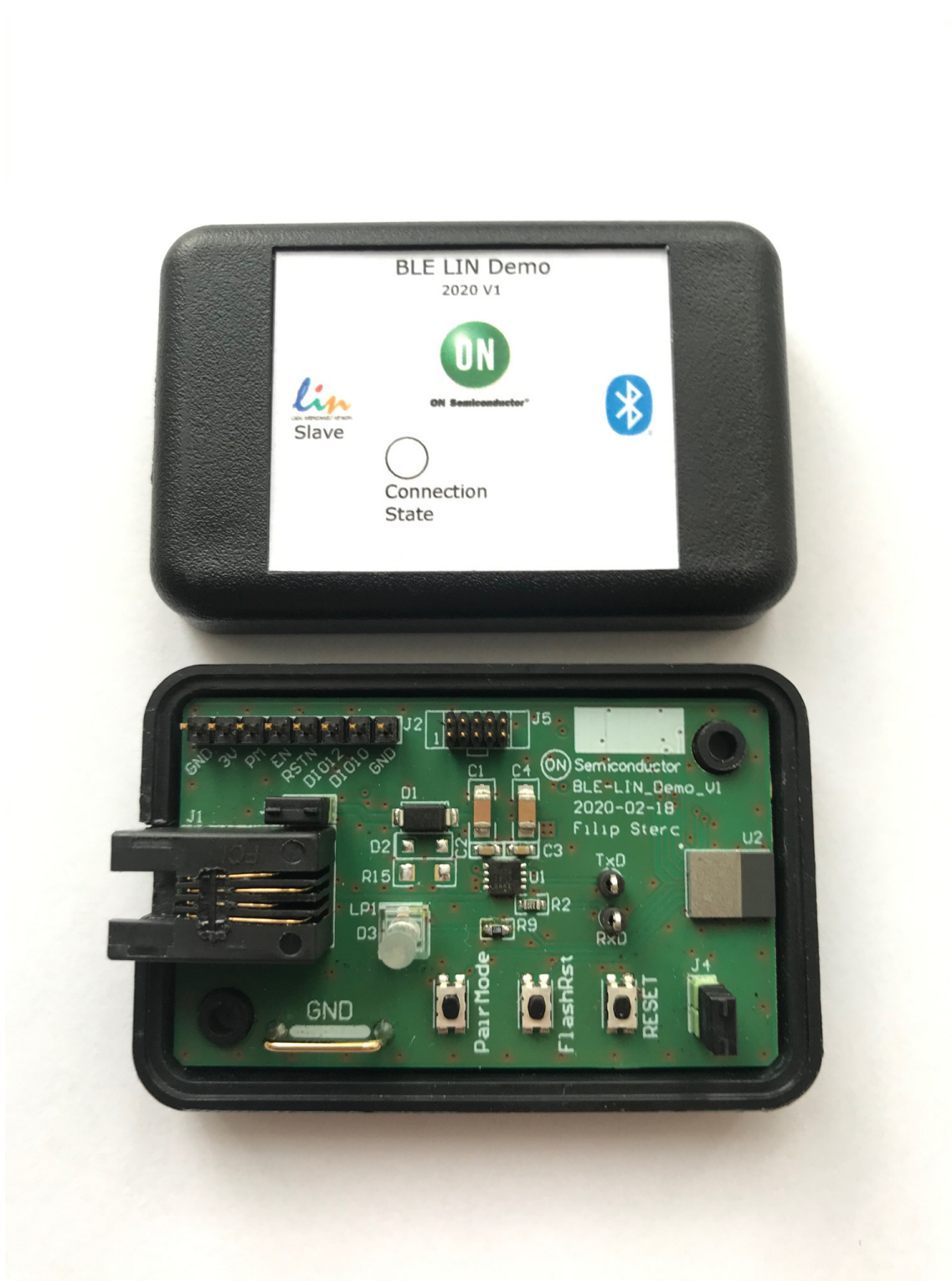
Fig. A.4: Picture of Keyless Entry module realization.
