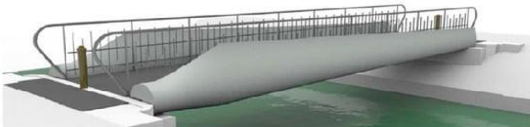
Figure A1. A conceptual design of a pedestrian bridge using part of A26 wind blades [44].
