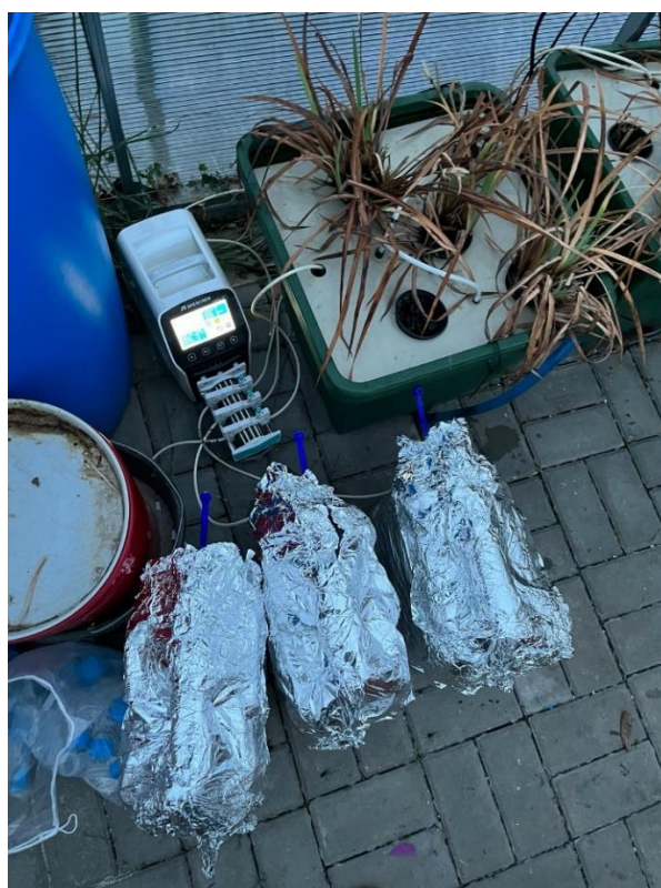
Figure n. 6 - Experiment setup with peristaltic pumps.
