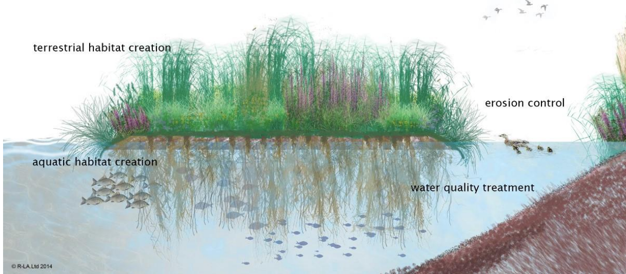
Figure n. 3- Design of floating treatment wetland (FTW) (Midwest Floating Island LLC, 2014)
