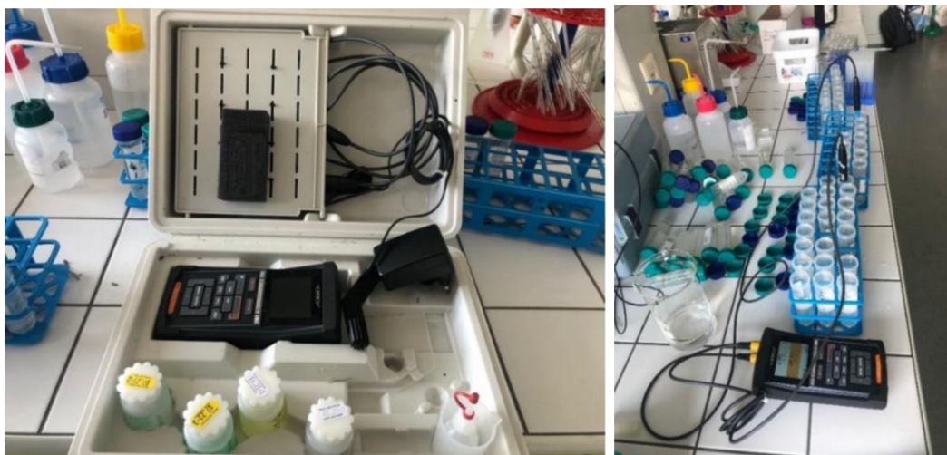
Figure n. 9-multi-parameter device Multi 3620 IDS SET C / Determination of pH and conductivity of water samples.
