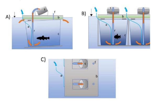
**Fig. 4: Schema of the pontoon monitoring device.** Side (A), front (B) and top (C) view. The device consists of these parts: a – air delivery hose, b – floating board, c – cage (individual tank), f – feeding port, r – rising pipe, s – filter cup. Arrows portray airflow (blue) and water flow (orange). Adapted from Douda et al. (2020).
