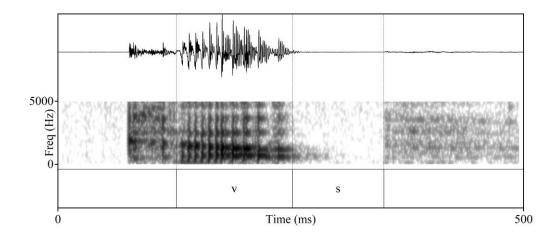
Figure 6: Segmented realisation of the manipulated neutralised target word *cup* by the native speaker. v = vowel /A/, lasting for 125 ms, s = voiceless consonant /p/.
