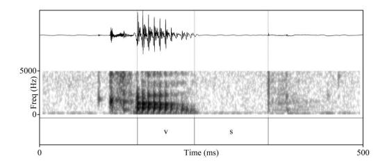
Figure 10: Segmented realisation of the manipulated native-like target word *cup* by the non-native model speaker. v = vowel / A / asting for 88 ms, s = voiceless consonant /p/.
