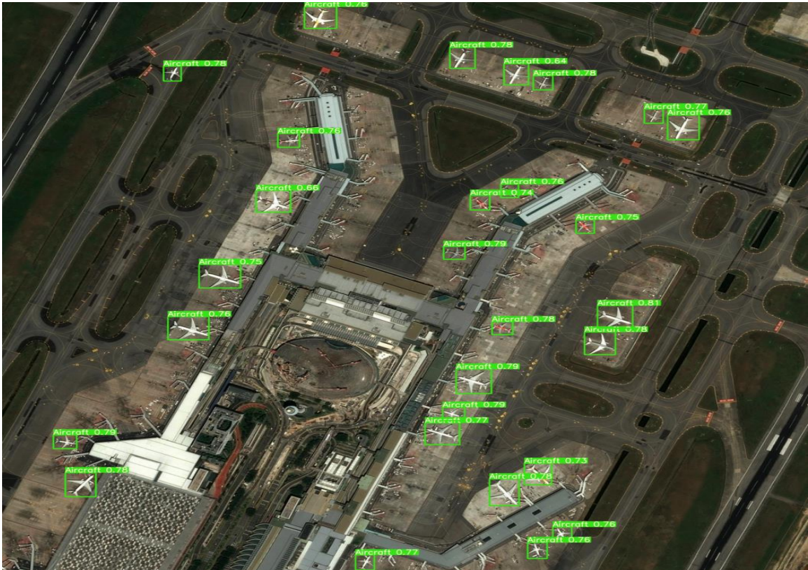
Figure 1. This image serves as an illustration of object detection. It depicts an airport scene with several airplanes parked, and through object detection, the system can identify the presence of these planes. Utilizing an AI system trained for aircraft recognition and based on the YOLOv7 algorithm – Built on Viso Suite https://viso.ai/deep-learning/object-detection/
