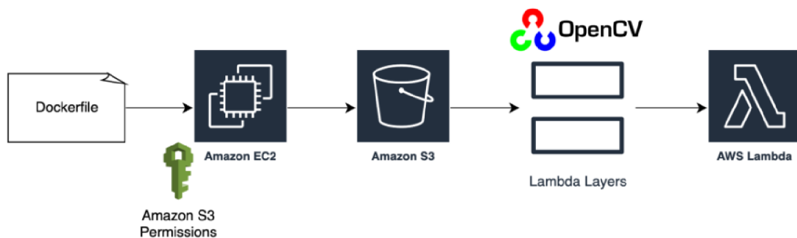
Figure. 19: Display that dockerfile deploy into the lambda function using S3 bucket resources and Ec2 Processing
