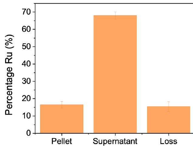
Figure 4.7: Loading of Ru-complex to DNA origami nanoblocks: pellets (Ru-complex-loaded DNA origami nanoblocks), supernatant (unbound Ru-complex) and the estimated sample loss [author].
