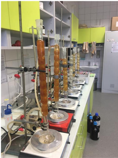
Figure 36. Set of reverse coolers for saponification value analysis.
