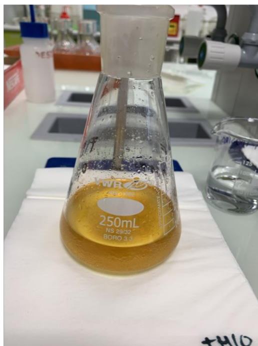
Figure 31. Peroxide value sample after first titration by solution \text{Na}_2\text{S}_2\text{O}_3 .
