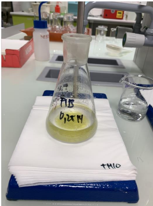
Figure 33. Final look of the peroxide value sample after second titration by solution \text{Na}_2\text{S}_2\text{O}_3 .
