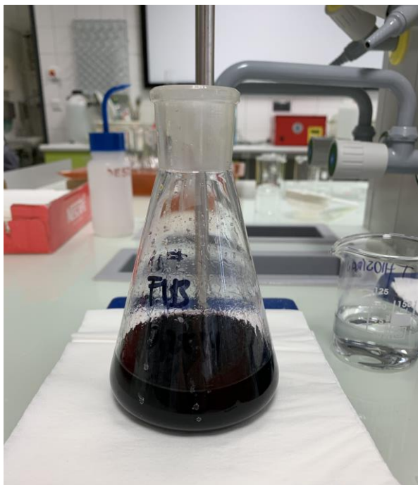
Figure 39. Iodine value sample with added colour indicator- starch.
