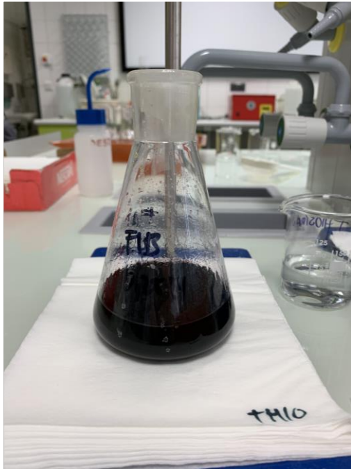
Figure 32. Peroxide value sample after adding colour indicator- starch.
