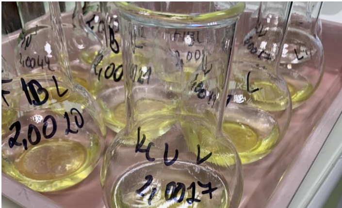
Figure 34. Acidity value oil samples with added neutralized ethanol.
