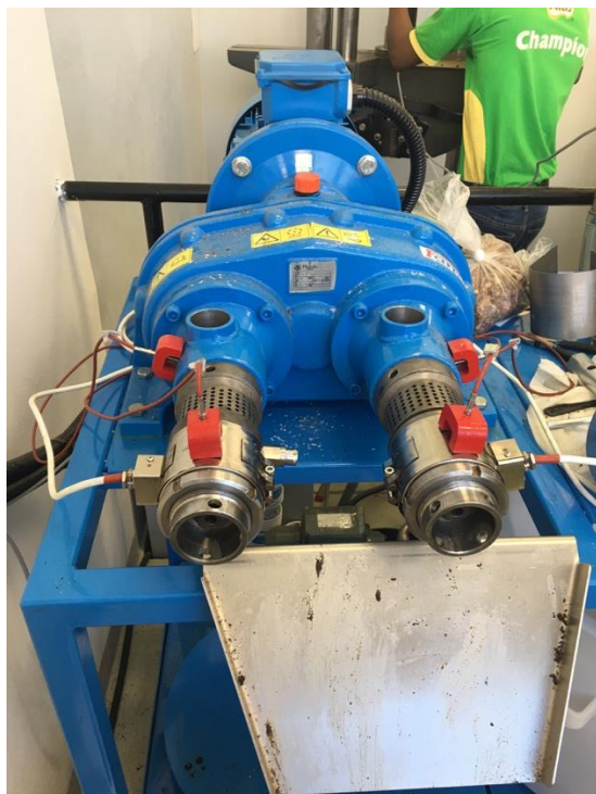
Figure 4. Mechanical crusher used for oil extraction (Author 2018).
