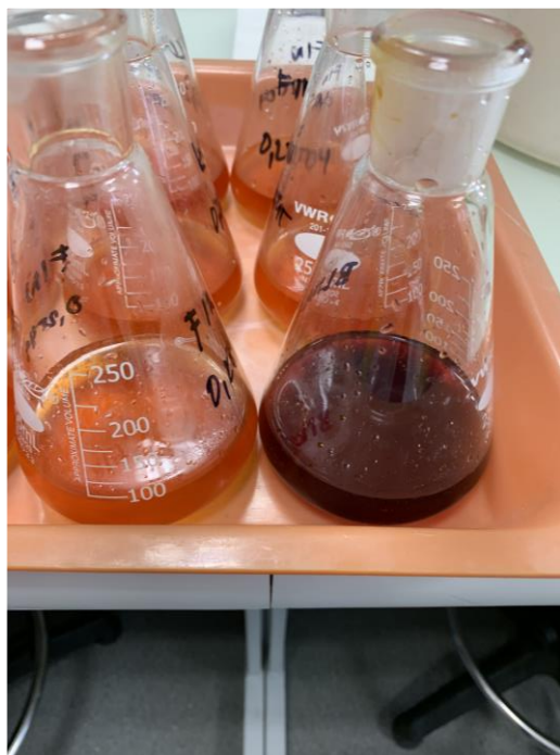
Figure 30. Prepared samples for obtaining peroxide value. State before first titration by solution \text{Na}_2\text{S}_2\text{O}_3 .
