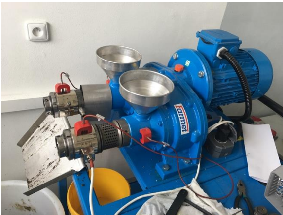
Figure 3. Mechanical crusher use for oil extraction (Author 2018).
