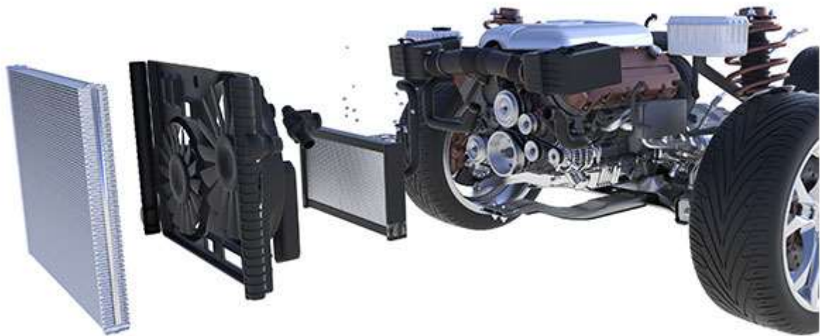
Figure 7 Schematic illustration of compact cooling module [43]
