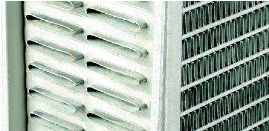
Figure 8 Detail view on the radiator core construction [19]
