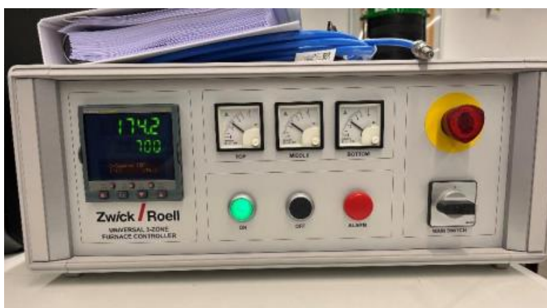
Obr. 52 Regulátor Zwick Roell Universal 3 zone furnace controller
