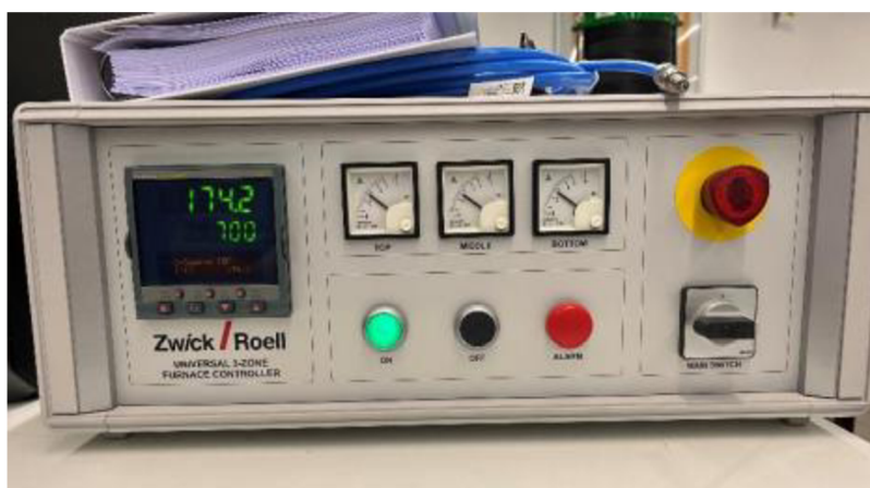
Obr. 52 Regulátor Zwick Roell Universal 3 zone furnace controller
