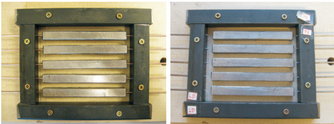
Fig. 2.5: A steel mould for the production of silicone forms.
