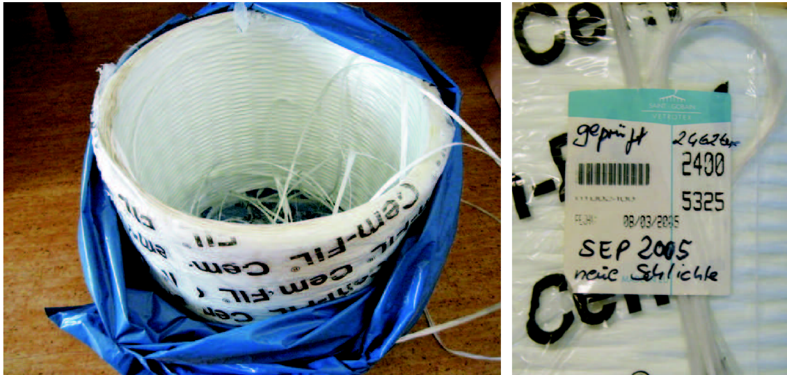
Fig. 2.1: The tested AR-glass yarn on a bobbin.
