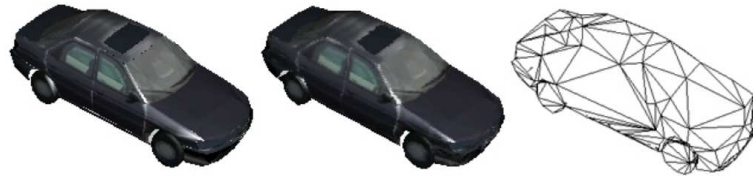
Figure 3.19: From left to right: original model, the texture depth mesh (TDM) representation and finally the mesh of the TDM 23 .
