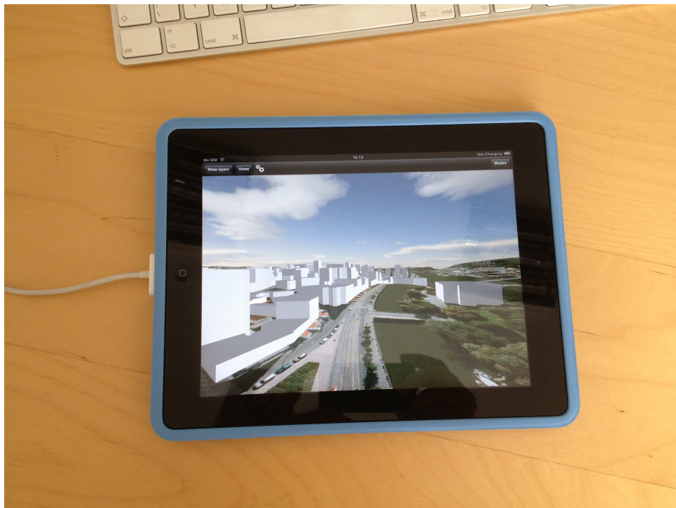
Figure B.1: Rendered terrain with buildings from user view on iPad 2 device. The data are streamed from remote server using the scheduling and prefetching mechanism proposed in this thesis.
