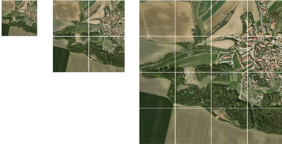
Figure 5.5: Part of the textures data pyramid which is created similarly as the elevation data pyramid.
