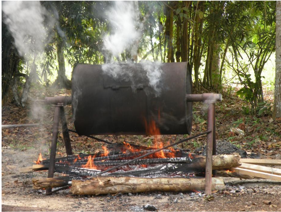
Photo 1: Biochar production system used at IIAP (Instituto de Investigaciones de la Amazonia Peruana) in Pucallpa for biochar production from rice husks. In this investigation it was used for biochar production from wood shaving. At IIAP charred rice husk is used mostly for vegetative propagation
