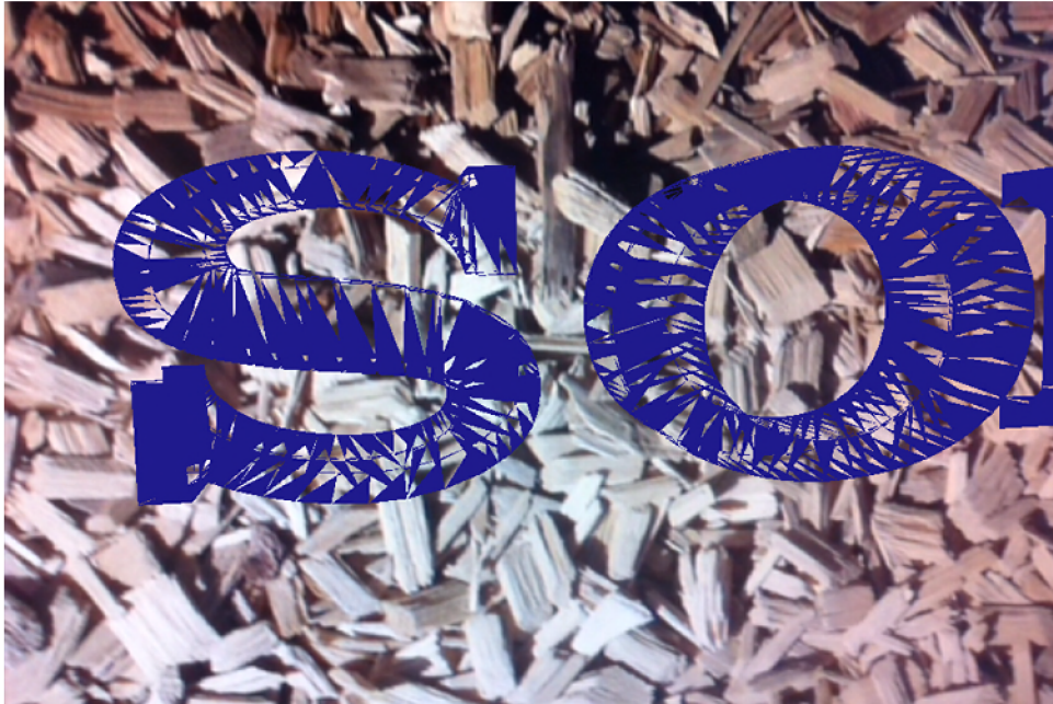
Figure 7-2: Demonstration of back-face culling problem
