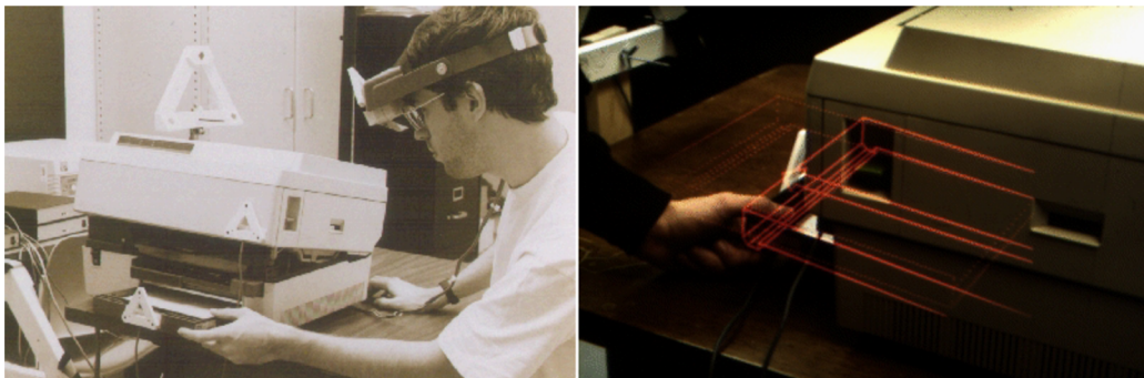
Figure 2-3: The printer maintenance program using AR [5]
