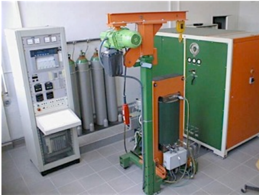
Obr. 22. HIP (ABRA Shirp, Switzerland)
