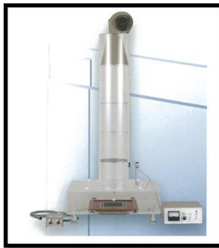
Figure 10. Image of wind column attached during measurement [69, 70].
