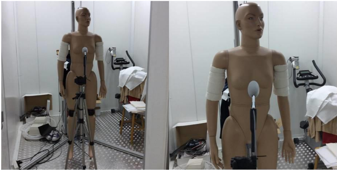
Figure 11. Image of P.T.Teknik thermal manikin, University of Lodz.
