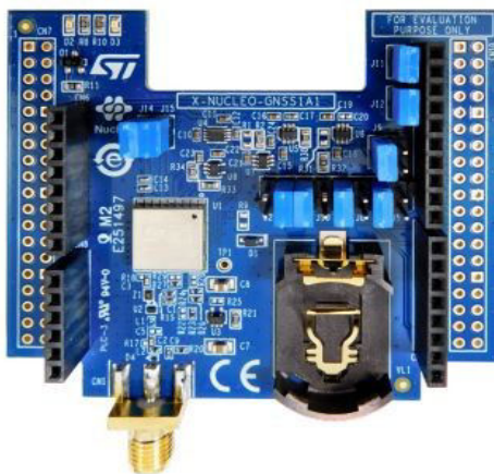
Obr. 3.14: GNSS prijímač X-NUCLEO-GNSS1A1 [8]
