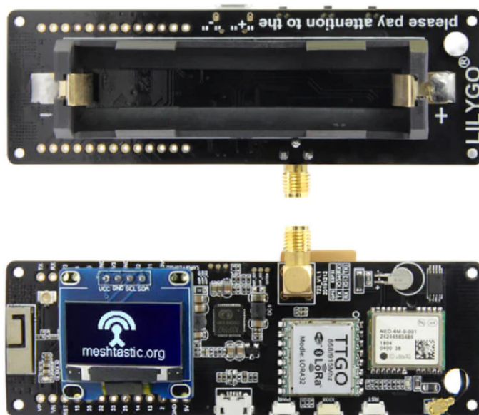
Obr. 3.5: Deska ESP32 TTGO T-Beam [45]
