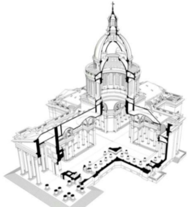
Figure 1: Axonometry of the Panthéon with cross-shaped floor plan and inside, (C. Blasi, E. Coisson, "The importance of historical documents for the study of stability in ancient buildings: the French Panthéon case study," vol. 7, no. 4, (Asian Journal of Civil Engineering (Building and Housing), 2006): 361).
