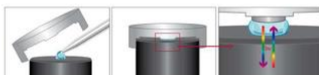
Fig. 2. Sample Compression Technology™ used in the NanoPhotometer™ Pearl.
