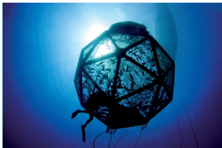
Fig. 9 An experimental version of an offshore towed fish cage with automatic feeding [33] (for license details see page 93)
