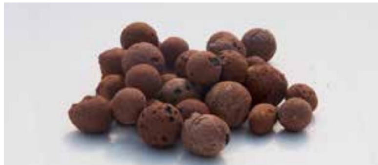
Fig. 19 Hydroponic growing medium: light expanded clay aggregate (LECA) [24] (for license details see page 93)
