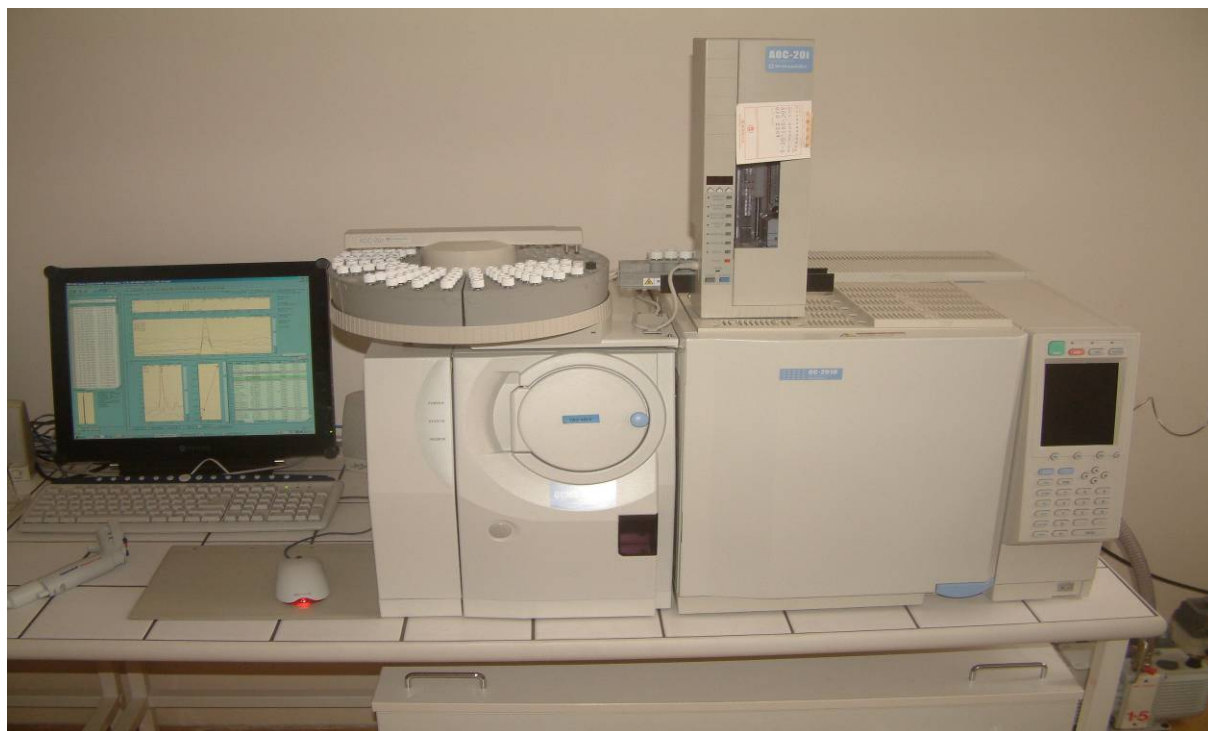
Obr. 10: GC/MS Shimadzu QP 2010
