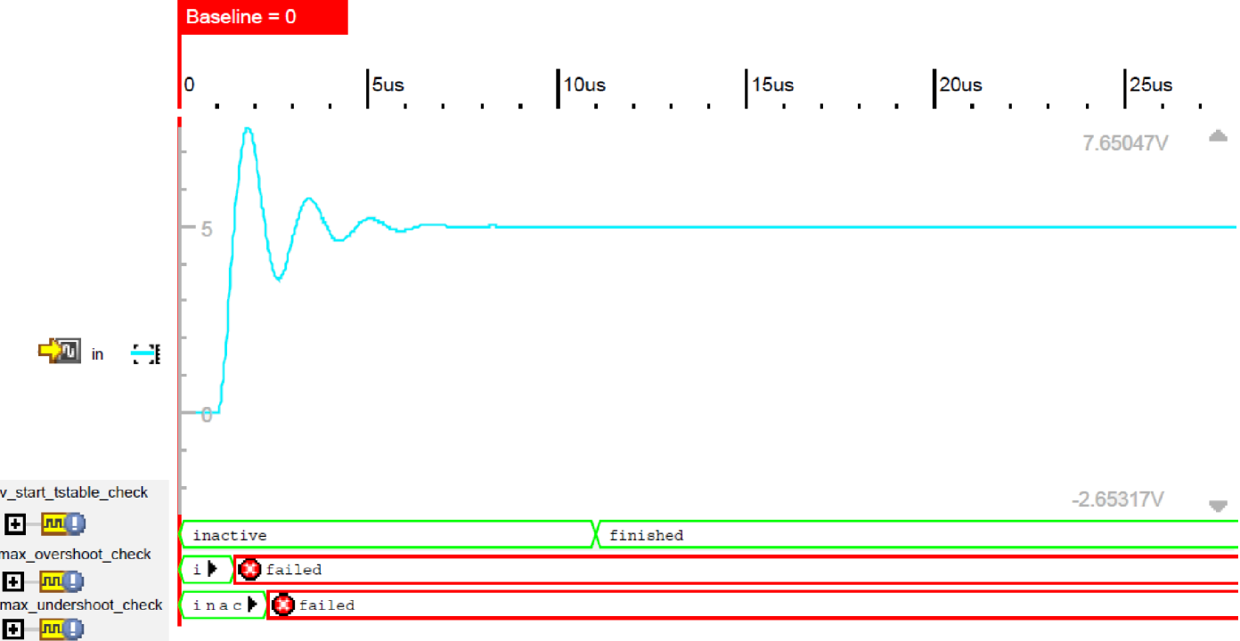
Figure 16: Voltage start-up assertion - second simulation result in Simvision.
