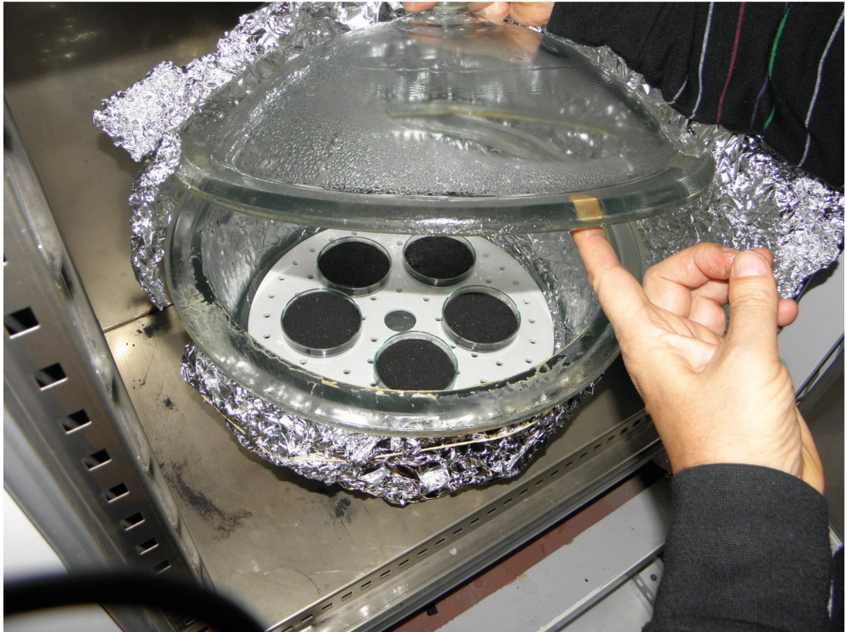
Figure 10: Measurement of sorption properties of samples by air humidity in the desiccator
