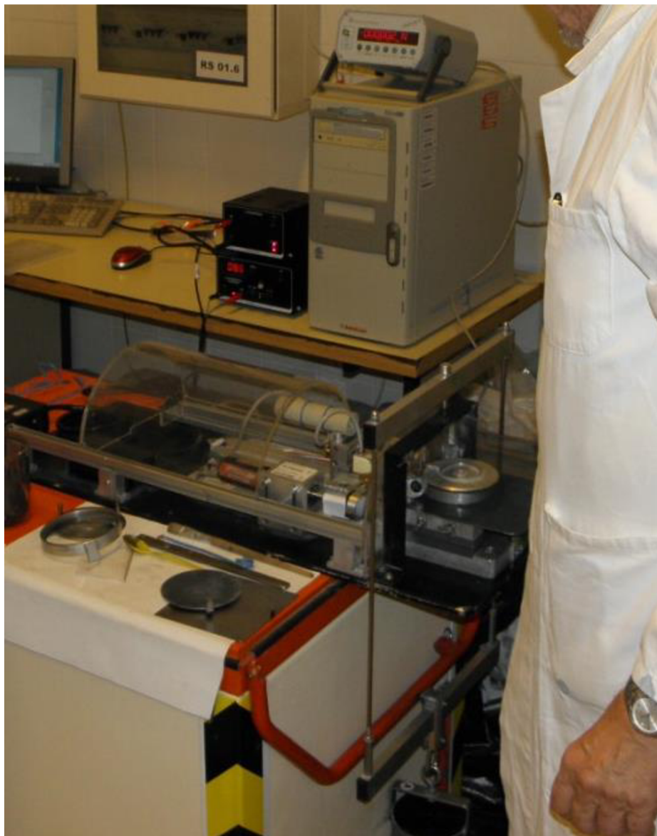
Figure 4: Measurement on Jenike shear device
