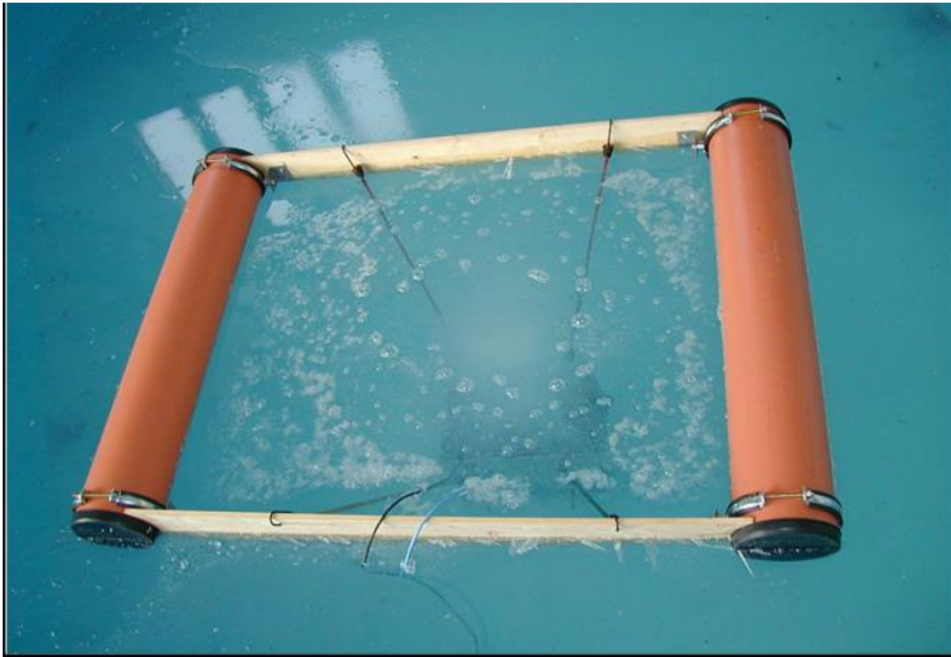
Figure 25: Electrocoagulation in full operation / loosening coagulation media
