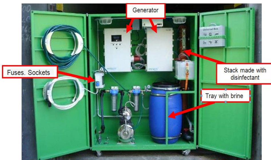
Figure 27: General view - a module for the production of disinfectant Vert Esprit
