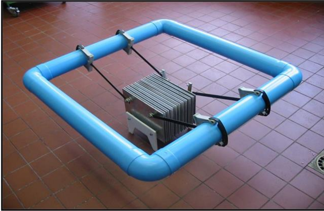
Figure 23: Construction of floats and reactor
