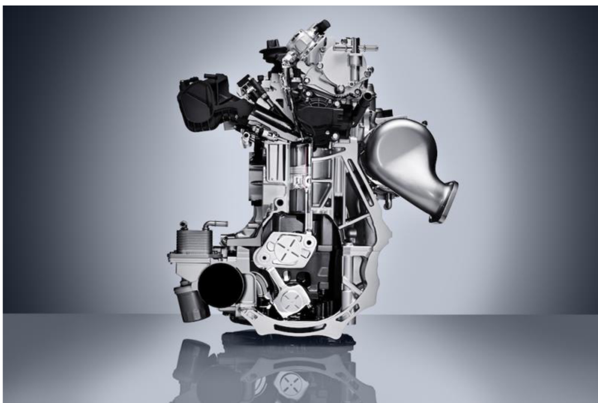
Obr. 9 - Rez motora Infiniti 2,0 VC-T [10]
