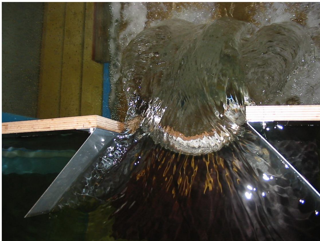
Obr. 5.8 Modelová varianta 4, h = 146 \text{ mm} , L/R = 1,57 , R = 141,5 \text{ mm} , pohled shora
