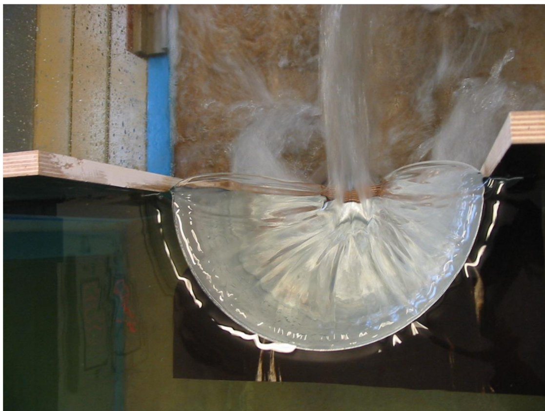
Obr. 5.3 Modelová varianta 2, h = 27 \text{ mm} , L/R = 3,14 , R = 150 \text{ mm} , pohled shora
