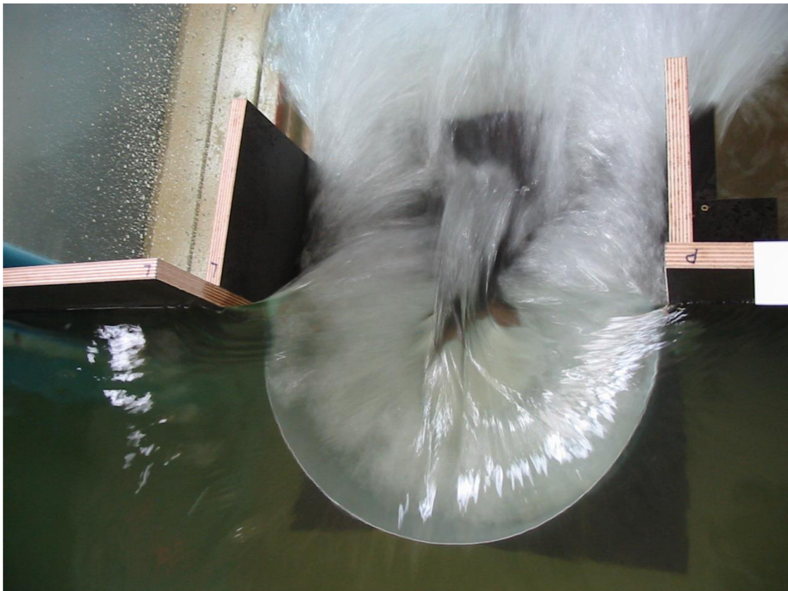
Obr. 5.6 Modelová varianta 3, h = 105 mm, L/R = 3,14 , R = 200 mm, pohled shora
