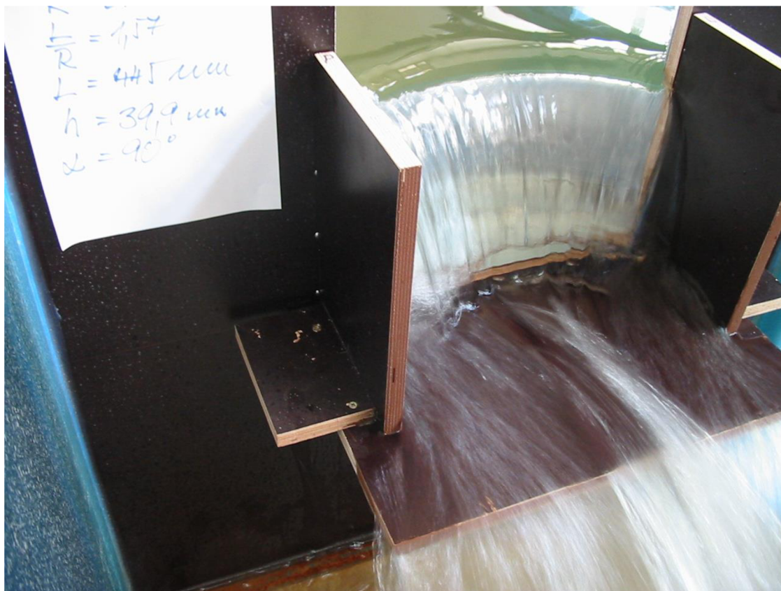
Obr. 5.13 Modelová varianta 6, h = 39,9 \text{ mm} , L/R = 1,57 , R = 283 \text{ mm}
