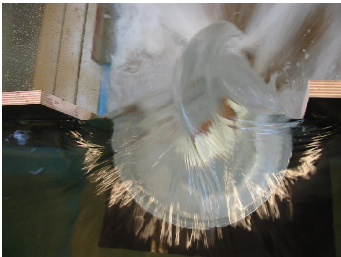
Obr. 5.4 Modelová varianta 2, h = 114 \text{ mm} , L/R = 3,14 , R = 150 \text{ mm} , pohled shora
