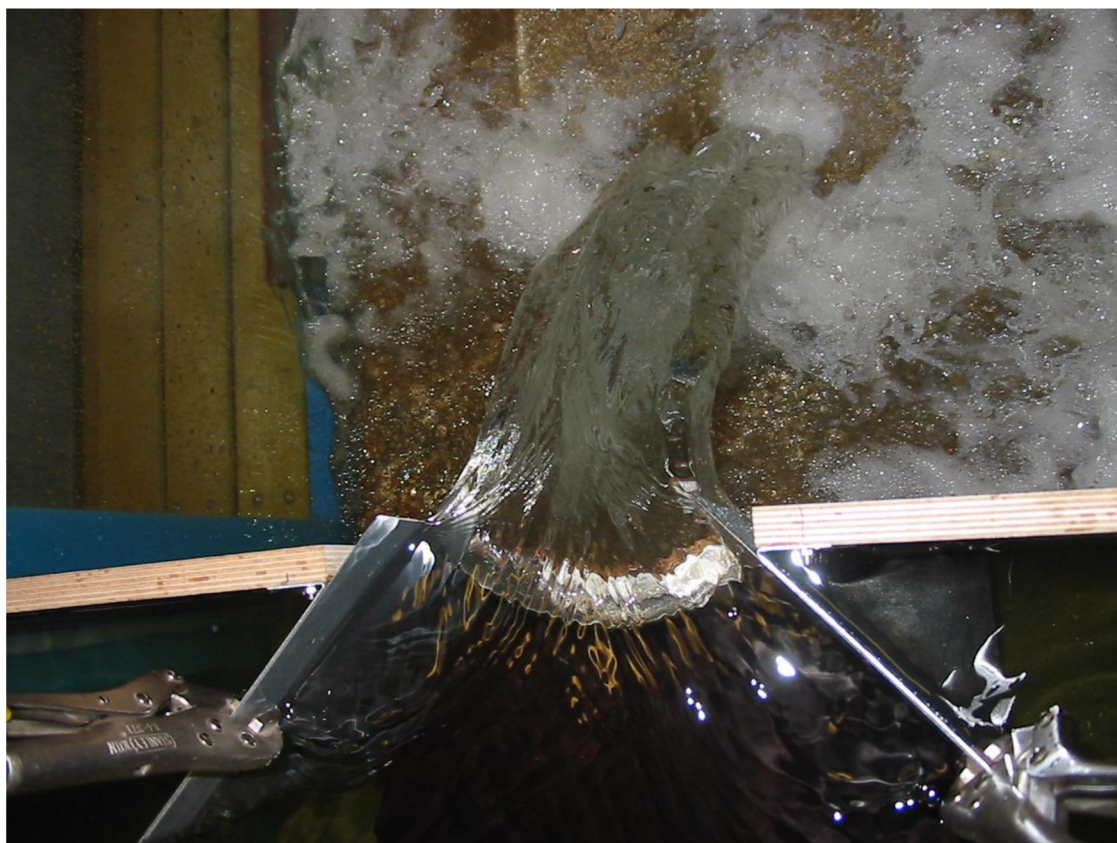
Obr. 5.9 Modelová varianta 4.1, h = 161,5 mm, L/R = 1,57 , R = 141,5 mm, pohled shora
