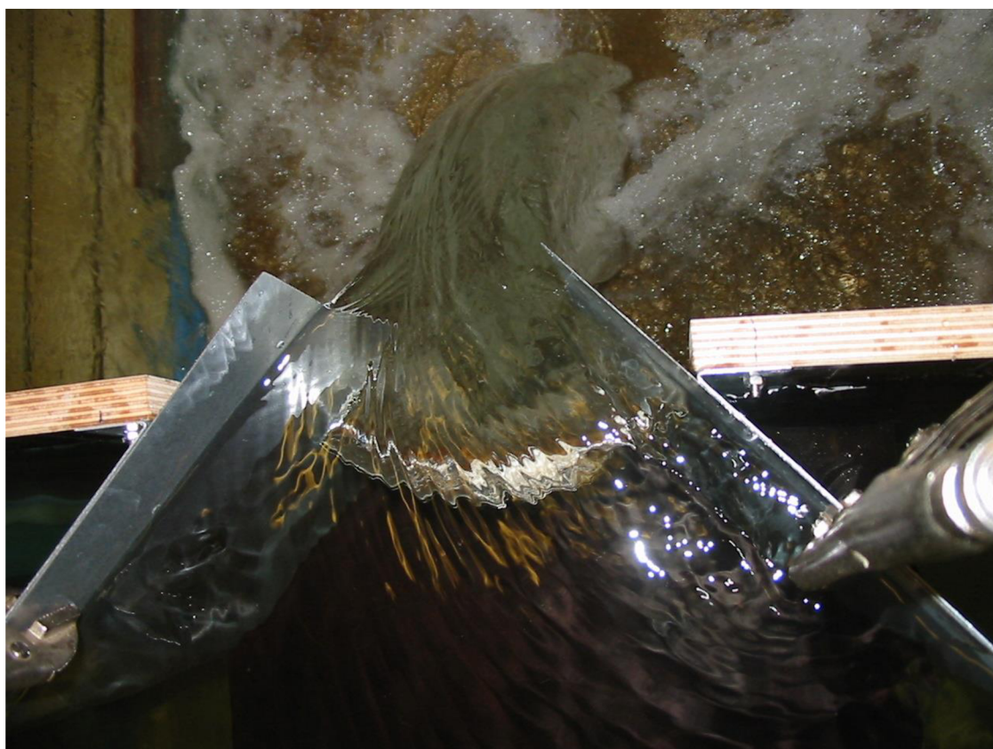
Obr. 5.10 Modelová varianta 4.2, h = 148,9 mm, L/R = 1,57 , R = 141,5 mm, pohled shora
