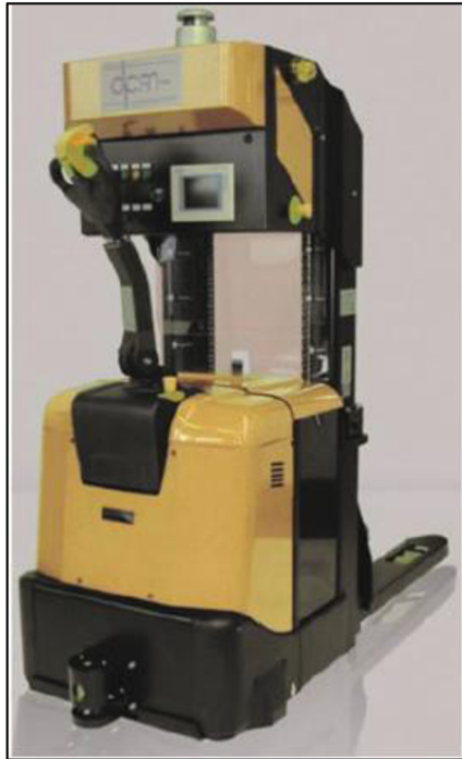
Figure 8: The forklift AGV, based on serially produced equipment [10]
