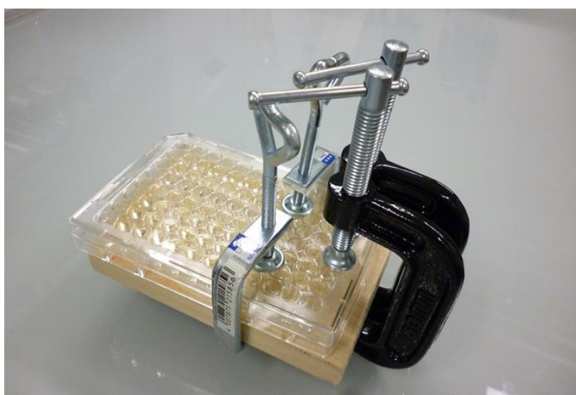
Picture 4. Fixed microtiter plate on a wooden plate
