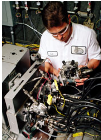
Fig. 11. Wear test of a fuel pump [15]
