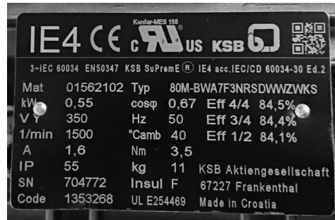
Figure 1.8: Reference SynRM label
