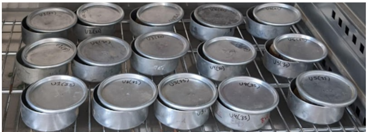
Figure 25 Soil from Sampling Rings in Metal Tins for Oven Drying (Source: Author).
