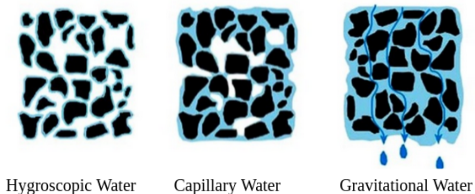
Figure 2 Diagram of the Different Types of Soil Water (Source: TerraGIS. Accessed 2024).
