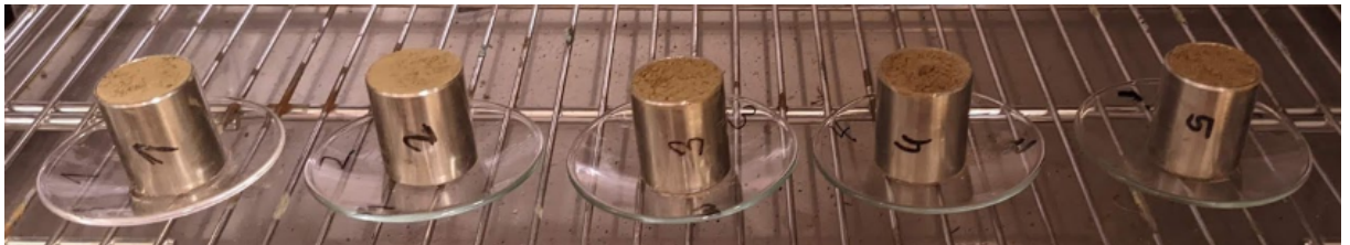
Figure 24 Sampling Rings with Watch Glass in the Oven (Source: Author).
