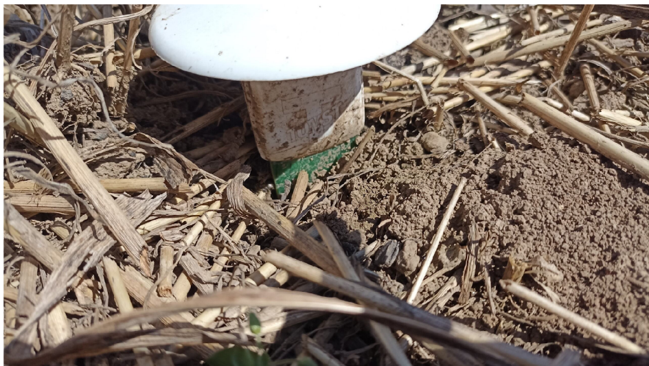
Figure 68 TMS-4 in Experimental Field Partially Uncovered from Erosion (Source: Author).
