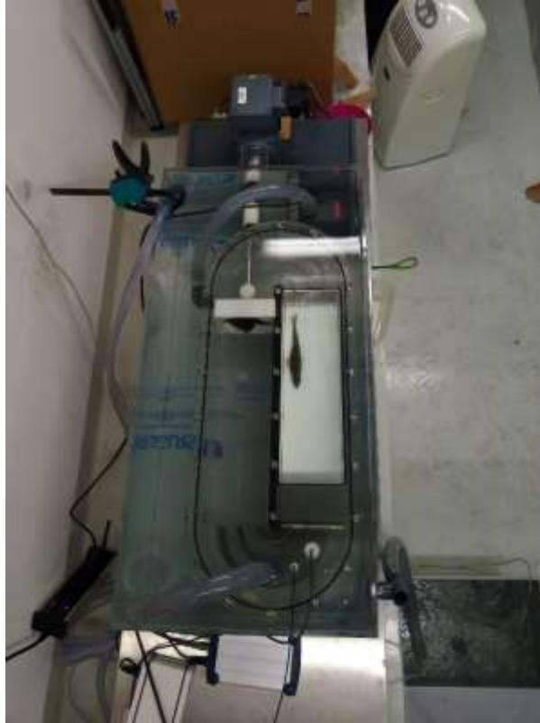
Fig 11. Top view of swimming tunnel with European perch during measurement
