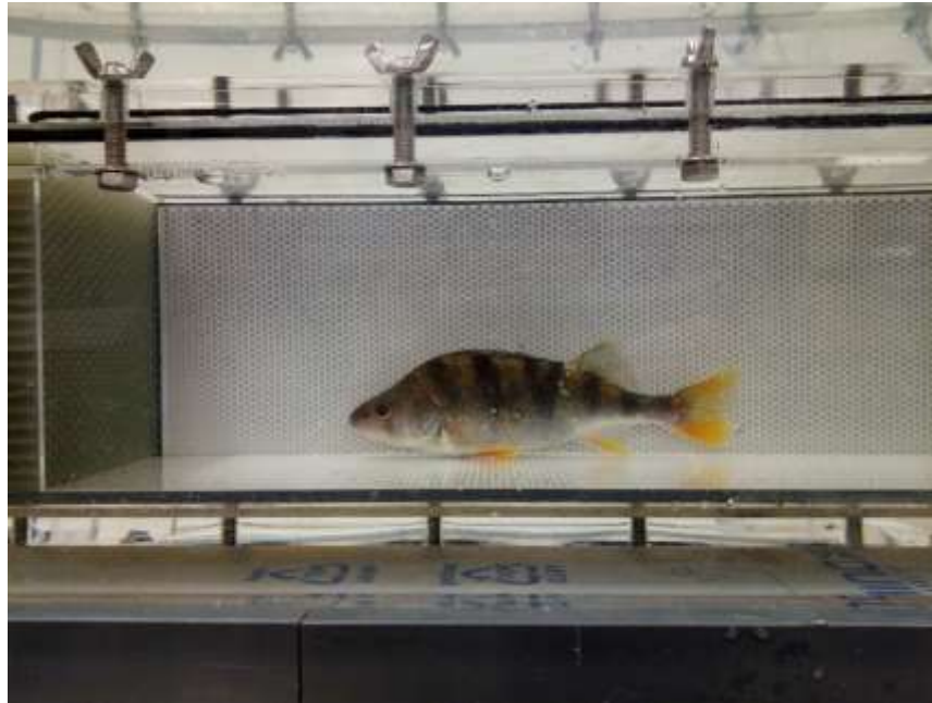
Fig 13. Detail view of European perch in test section (cabine) of swimming tunnel during measurement
